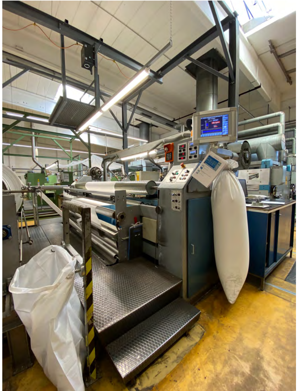
Fig. 3: The Famacont PMC integrated in the production line
